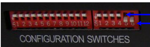
Figure 2 Auxiliary DIP switches
