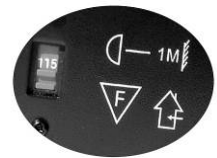
Figure 1 - AC Voltage Switch
